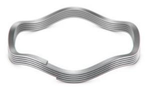
Such wave springs cannot be calculated with FED14. In FED14, the number of waves is 2.5, 3.5, 4.5; here it is 3.0, 4.0, 5.0. Such wave springs can only be calculated with FED13, or with FED14, one coil (n=1.0), then the spring force multiplied by the number of coils n. This is analogous to layered disc springs with FED4.
